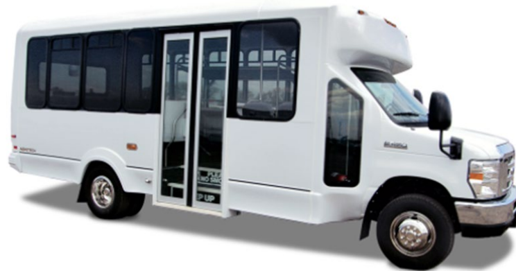
Example of an electrified Paratransit bus, built on a Ford E-450 chassis. a 127kWh battery; 105 mile range https://www.motivps.com/application/electric-shuttle-bus/
